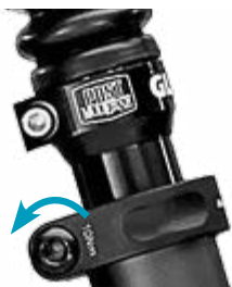
For 1. Loosen the saddle clamp bolt(s)
