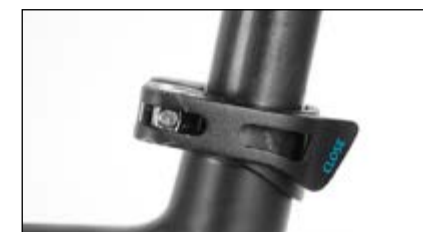
For 3. Quick-release skewer closed
