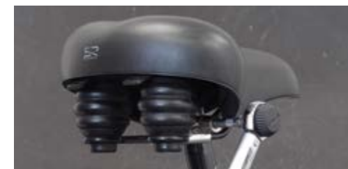
For 1. Loosen clamping nut
