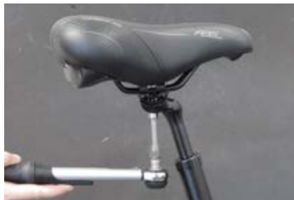
For 1. Loosen the clamping screw
