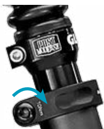
For 3. Tighten the saddle clamp bolt(s)
